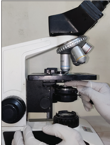
Figure 2: Correct placement of the coin beneath the condenser.
